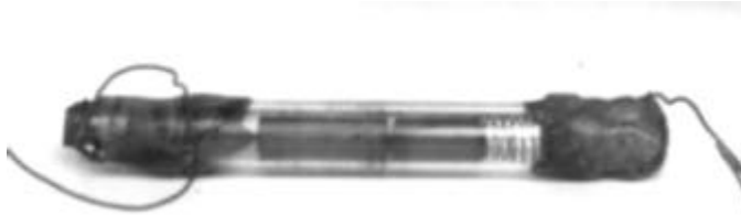
Figure 4. A cylindrical microphone developed by Hughes, including a loosely contacted carbon cylinder with loose filings inside the tube. Note the similarity to later Branly and Lodge coherers. Hughes abandoned this as a detector of electromagnetic waves because it did not self-restore. (Science Museum, London)
